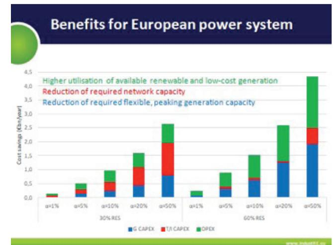
This graph illustrates how 1,5 b€/year could be saved if 10% of the industrial demand becomes flexible, through higher utilisation of RES and reduction of required peaking generation capacity.
